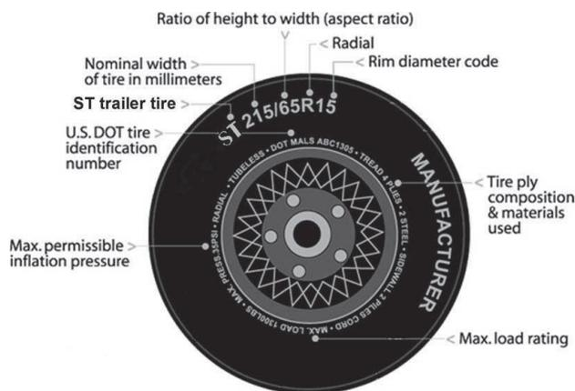
**Maximum Permissible Inflation Pressure:** Indicates the tire manufacturer’s maximum permissible pressure and/or the pressure at which the maximum load can be carried by the tire. Refer to the Certification Label on the port forward half of the trailer for the correct tire pressure for your trailer.
