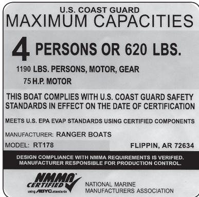
Familiarize yourself with your boat's maximum capacities. Do not exceed the maximum weight (in pounds) or persons capacity (number) found on the U.S.C.G. capacity information plate attached to your boat. **Know the ratings and load your boat accordingly. It is a must for safe boating.**
