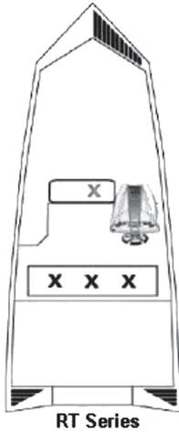
**! WARNING** Do not operate the boat on plane with persons located outside the on-plane seating locations shown on the decal. Failure to do so could cause a person(s) to be thrown overboard resulting in injury or death.
