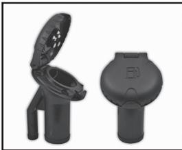
Periodically inspect the deck fill plate for damage. Be sure to use the exact fuel fill/vent used on your boat if replacement is required. Excessive pressure or vacuum in the fuel tank may damage the fuel system, if cap is substituted. (Fuel fill deck plate is not waterproof; water can be drawn into fuel tank during vent operation, if fill is submerged.)
